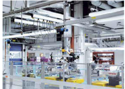
Rail system for components handling unit or manipulator
